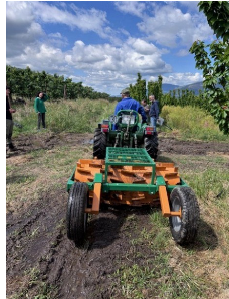
Showing the use of roller crimper. Source: Cherry Spain
